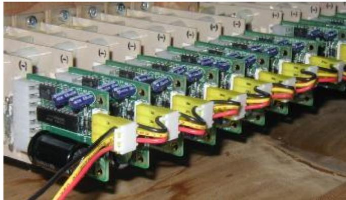
Daisy Chain Cable installed on SC units on a stop rail
