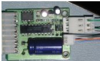
The above photo shows the small 3 pin programming plus attached to the SC. The SC may now be programmed.
