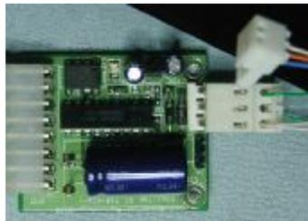
The above photo shows connection of the large 3 pin header to the SC to be programmed.
