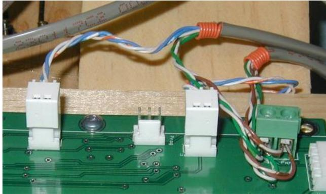
Note that there is no operational connection to be made to the “Prog” header.
