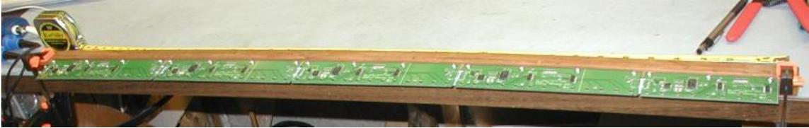
The above image shows 5 modules mounted to a Wurlitzer contact rail, ready for mounting in a keyboard.
