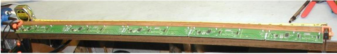
Here is a close-up of the bass end of the keyboard sensor. This side is the one that will go towards the magnet holders. Normally the magnet holders are attached to the underside of the keys and key movement will move the magnet towards the sensor. The individual sensors are the small block rectangles near the outer edge of the circuit card.
