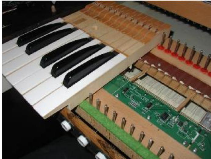
Here the sensors have been mounted to the front keyboard support rail. The magnets are installed in small 1/8 x 1/8 holes drilled into the bottom of the keys.
