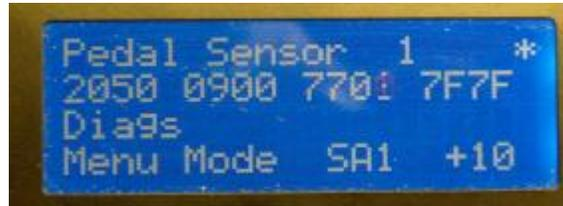
The Diag screen is a quick way to look at any given sensor to check operation.
